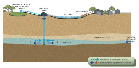
The ASR Scheme, located in the Mernda Villages' vast wetlands, allows large quantities of water to be stored without evaporation and with reduced risk of contamination from pollutants, both of which are problems associated with surface water storage areas such as reservoirs and dams.
