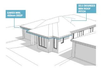
Where the design is contemporary and does not allow for any eaves, the use of awnings and/or sun shade materials is strongly encouraged where there is a window to improve energy efficiency.
