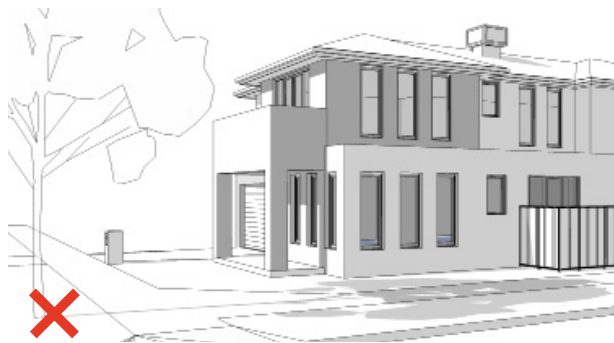
Non compliant evaporative cooler unit located at side of roof and above roof ridge line
