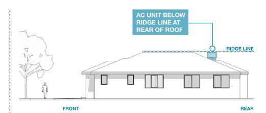
Evaporative Cooler Units must be placed below the roof ridgeline at the rear of the roof
