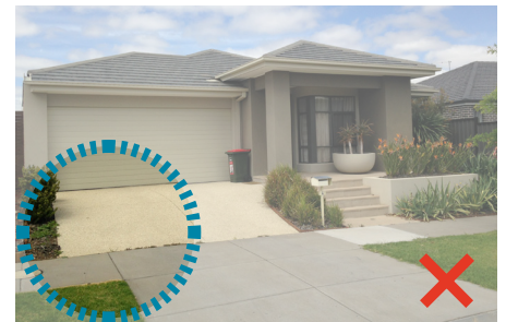
Driveway does not align with crossover
