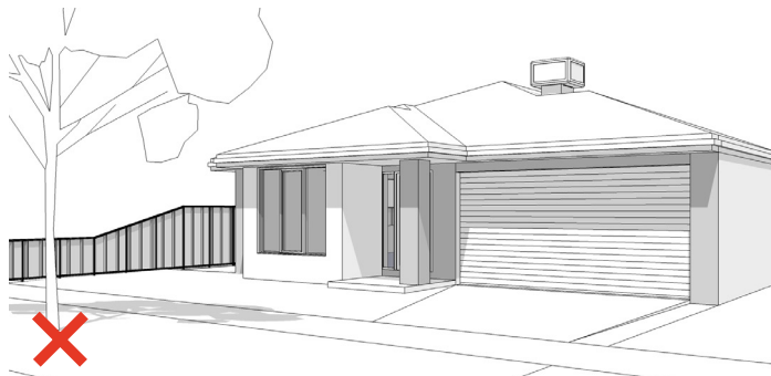
Non compliant evaporative cooler unit located at front of roof and above roof ridge line
